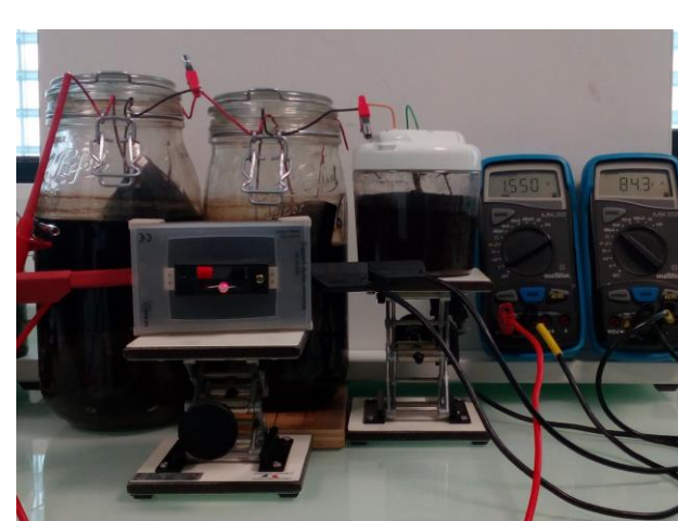
Serial association of 3 MFC's to power on a LED (1,35 V, 100 μA)
